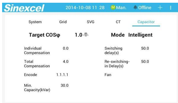
Figure A- 62 Capacitor settings information
