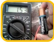
Even though multimeters have their own revisions Schedule, it is convenient to verify it works properly, specially to check voltage absence. It could be damaged and show incorrect values. Use a 1.5V battery to verify proper functioning.
