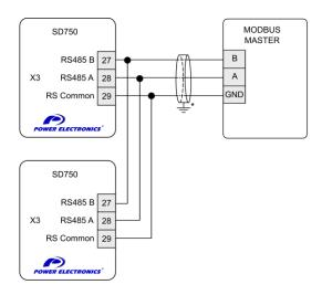
\* Screen connection must be performed on the side of the Modbus master or on the other side depending on the installation. SD75DTR0002CI It is recommended to connect the jumper "RS485 USER" at the first and the last device of the RS485 communication network, to connect the end of line resistor.
