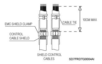
Cable shields for digital signal must be grounded at both ends of the cable. It is recommended to use independent shielded cables for digital and analogue signals. When using multiple analogue signals, do not use common return for them. If using analogue signals, a low interference is experienced (hum loops), disconnect the shield grounding from one of the ends. The maximum section for the control cables is 2.5mm<sup>2</sup> and the recommended tightening torque is 0.4Nm.
