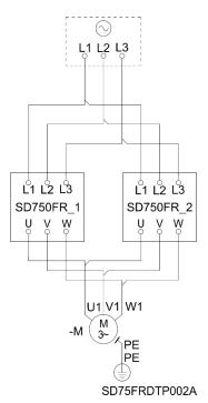
Power wiring connection for variable speed drives composed of two equipment of frame 9 to 11
