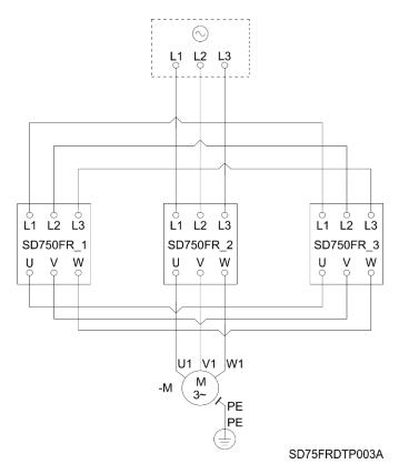
Power wiring connection for variable speed drives composed of three equipment of frame 9 to 11
