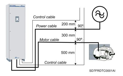
Power Electronics recommends installing separately the following circuits, whether in cable racks, trays or in different wire ducts:
