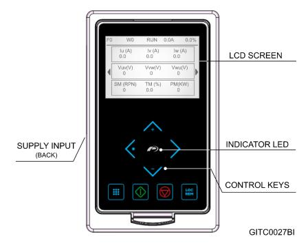
The LED indicator generates three different colors depending on the status of the drive, which indicates the following information:
