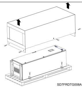
To unpack, if necessary, unscrew the screws that fix the wooden box to the pallet. Then, unscrew the fixing screws on the angle brackets. To lift the drive and place it in a vertical position, use only a crane or a forklift equipped with straps or slings. Lift gently by pulling the top bolts.
