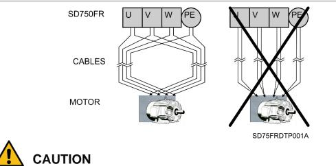
Line voltage (input supply) must never be connected to U, V and W terminals. Otherwise, the drive may get be damaged.
