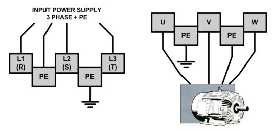
The input and output busbars are labelled according to the following diagram.
