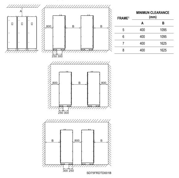
**Note:** It is recommended to have enough space in the front side of the equipment. The distance must be higher than the minimum distance in order to be able to move the equipment in case of need.
