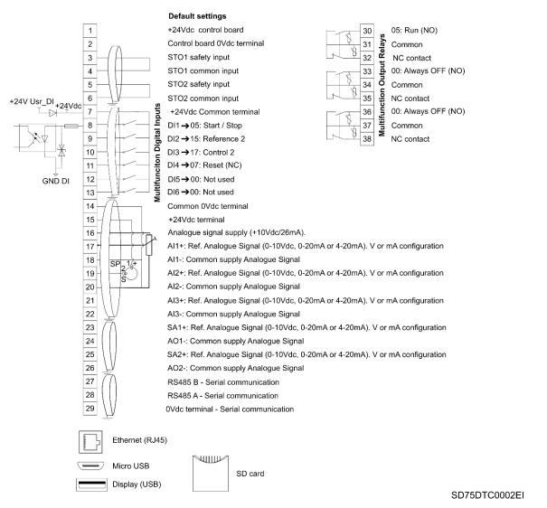
Digital inputs can be configured individually or collectively. Analogue inputs can be configured as comparators. For further information on configurations, please refer to the *Software and Programming Manual*. The following figure shows the wiring detail of the X1 connector with the wiring of the three-wire start / stop buttons.
