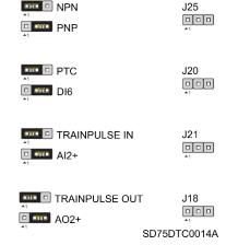
Positions Jumper (Signal) Description 3 AO J18 (AO2+) Configures AO2+ as Analogue Output or Pulse Output. 2 Pulse output 1 D 3 DI J20 (DI6) Configures the AI6 as Digital Input or PTC. 2 PTC D 1 3 AI J21 (AI2+) Configures the Al2+ as Analogue Input or Pulse Input. 2 Pulse input 1 Ľ 3 PNP J25 (DI1 a DI6) Configures each DIx as NPN or PNP. 2 NPN 1
