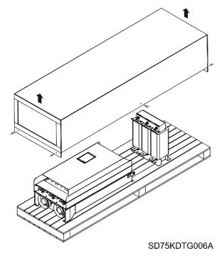
To unpack, if necessary, unscrew the screws that fix the cardboard or wooden box to the pallet. Then, unscrew the fixing screws on the angle brackets.
