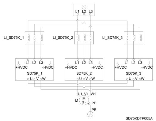
Connection of four modules must be made as shown in the following diagram.
