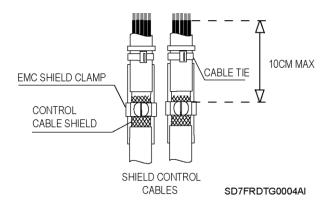
Cable shields for digital signal must be grounded at both ends of the cable. It is recommended to use independent shielded cables for digital and analogue signals. When using multiple analogue signals, do not use common return for them. If using analogue signals, a low interference is experienced (hum loops), disconnect the shield grounding from one of the ends. The maximum section for the control cables is 2.5mm² and the recommended tightening torque is 0.4Nm.
