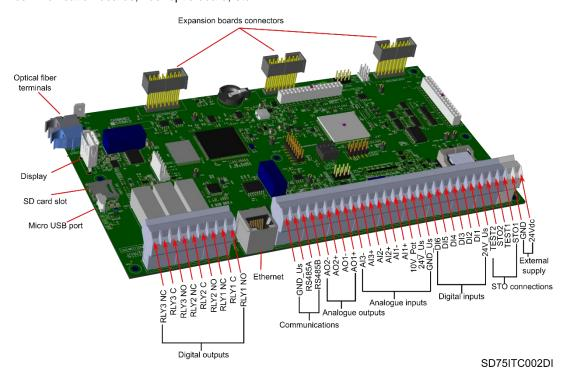
**Note:** Each expansion board connector is attached to a rack. The following table details, from right to left, the default position of each expansion board connector, with rack No. 1 being the rightmost and rack No. 3 the leftmost.
