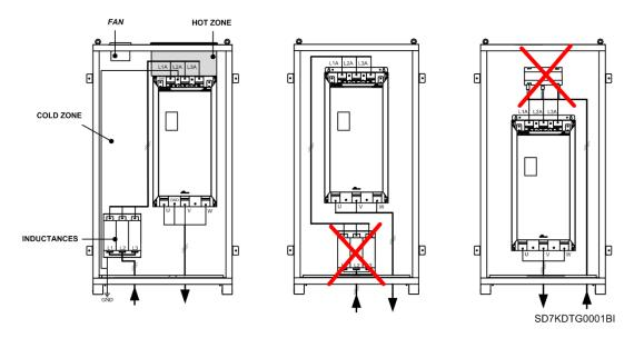
The cabinet must have two isolated zones, which permit independent cooling systems:
