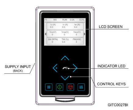
The LED indicator generates three different colors depending on the status of the drive, which indicates the following information:
