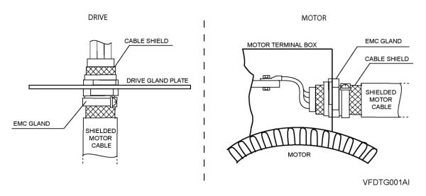
It is recommended to use shielded cable for control signals and to follow recommendations included in section "Wiring recommendations".
