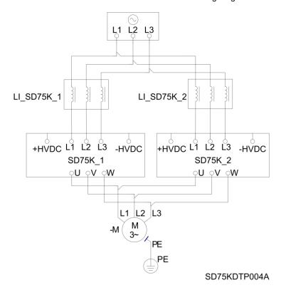
Connection of three modules must be made as shown in the following diagram.
