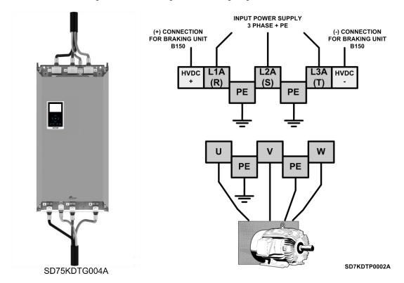
Note: It is recommended to use an earth cross section equal or higher than active wires cross section.
