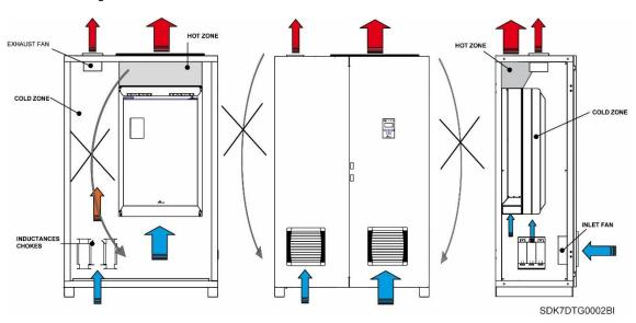
The IP54 cabinet must be equipped with the additional features:
