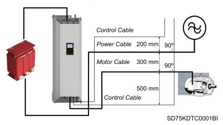
Power Electronics recommends installing separately the following circuits, whether in cable racks, trays or in different wire ducts:
