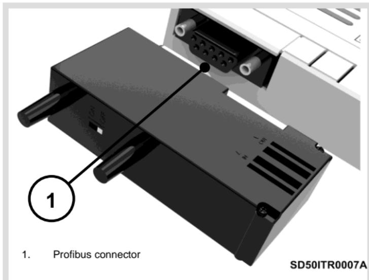
*Figure 3.3 Location of the connector on the Profibus board*
