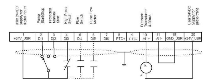
NOTE: the remote control cables must be screened
