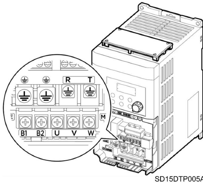
The motor chassis ground must be connected to the drive. In other words, connect the motor's ground conductor to the PE protection terminal of the drive and not to the installation's ground. It is recommended that the section of the motor ground conductor (PE) has at least the same cross section as the motor power cables sections (U, V, W). Additionally, it must be installed following the recommendations indicated in sections [Power connection and wiring](#).
