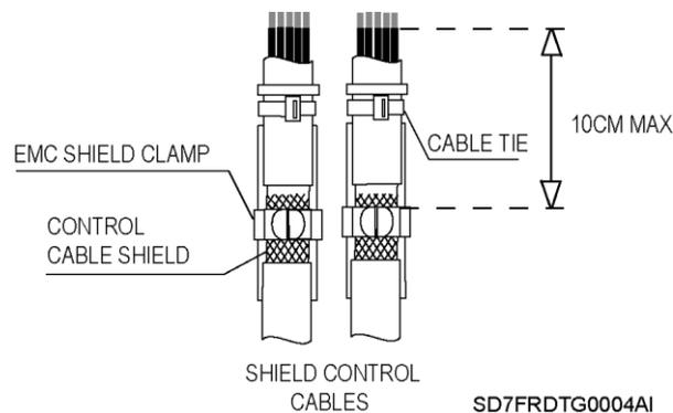
Cable shields for digital signal must be grounded at both ends of the cable. It is recommended to use independent shielded cables for digital and analogue signals. When using multiple analogue signals, do not use common return for them. If using analogue signals, a low interference is experienced (hum loops), disconnect the shield grounding from one of the ends. Refer to [Recommended cable section](#) for cable specifications and recommended adjustment.
