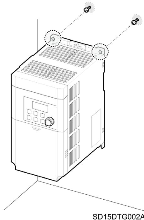
Mount the drive on the wall or inside the panel using the top two bolts and then fully tighten the mounting bolts. Ensure that the drive is placed flat on the mounting surface and that the surface can securely support the weight of the drive. Use the following image as a guide.
