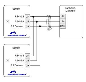
\* Screen connection must be performed on the side of the Modbus master or on the other side depending on the installation. SD75DTR0002CI RS485 connection It is recommended to connect the jumper "RS485 USER" at the first and the last device of the RS485 communication network, to connect the end of line resistor.
