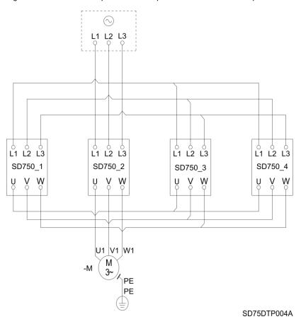
Power wiring connection for variable speed drives composed of four modules of 6 pulses frames 9 to 11
