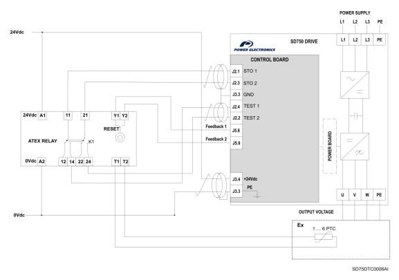
Connection scheme (Example with ZIEHL - PTC Thermistor Relay Type MSR 220 Vi)
