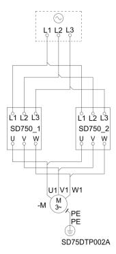
Power wiring connection for variable speed drives composed of two modules of 6 pulses frames 9 to 11
