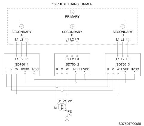
Power wiring connection for variable speed drives composed of three modules of multipulses frames 9 to 11
