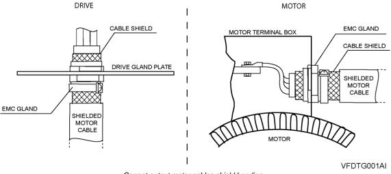
Correct output motor cables shield bonding
