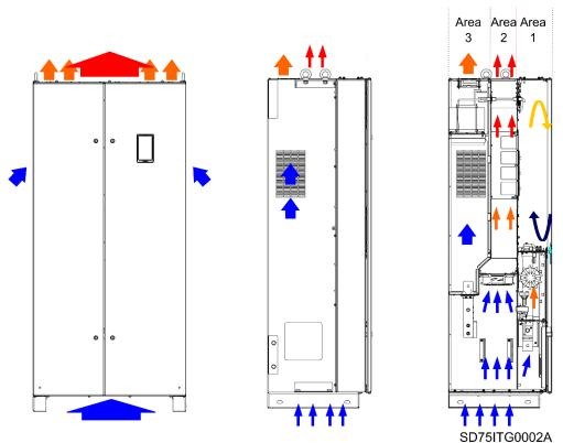
Cooling airflow for SD750. Frames 4 to 11(Protection Grade IP54).
