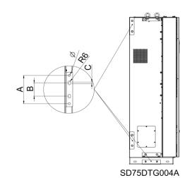
It is recommended to construct a cable duct to get the cables to the input / output connections. The duct width must not exceed 300 mm and the ground contact surface must withstand the weight of the cabinet that falls on its legs.
