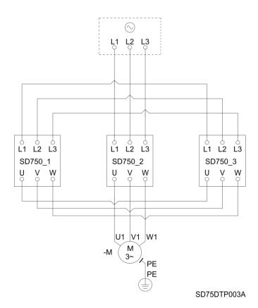
Power wiring connection for variable speed drives composed of three modules of 6 pulses frames 9 to 11
