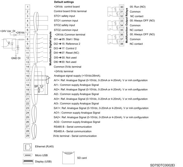
Example of control terminals standard wiring
