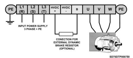
Power wiring connection for frames 1 and 2
