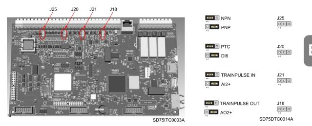
Location of jumpers in the control board (left) and connection detail (right)
