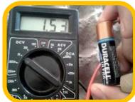
Even though multimeters have their own revisions Schedule, it is convenient to verify it works properly, specially to check voltage absence. It could be damaged and show incorrect values. Use a 1.5V battery to verify proper functioning.
