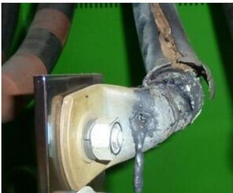
*A solder lug overheated by high harmonic currents has melted the solder in the lug.*
