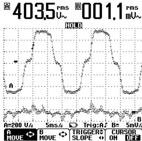
A voltage trace of a supply showing in excess of 15% THDV. This site was experiencing random electronics failures and unexplainable production outages.
