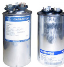
A “bulging” capacitor due to excessive heat versus it’s “normal” counterpart
