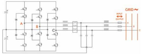
Innovative three level inverter circuit
