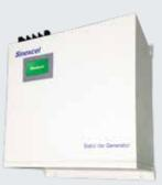
100kVAr Wall-Mounted SVG/ASVG 505W x 271D x 545H (mm) Weight: 62kg NOTE: Wall mount models are supplied with a top cover. Allow a further 150mm in height on 50kVAr model, 200mm on 100kVAr model and 300mm on 200kVAr model when using top cover.
